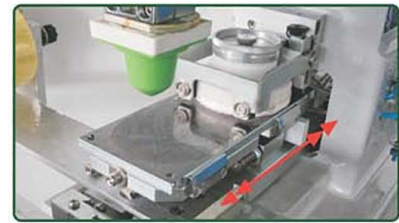
Platform in / out movement (Pad clean underneath)
